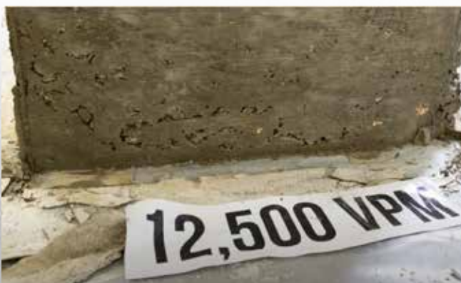
12,500 VPM - Poor consolidation and finish
